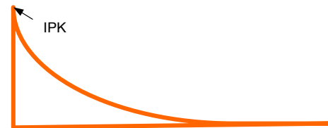
Figure 26. Input Charge Inrush Current
